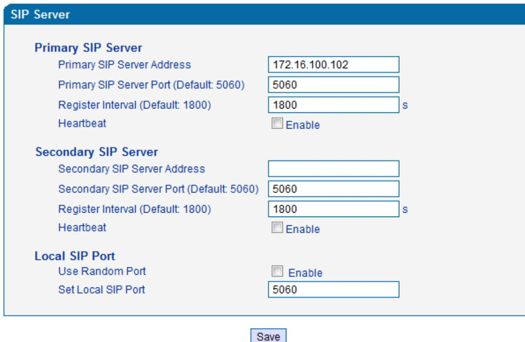
Figure 4.6-1 SIP Server Configuration Interface
